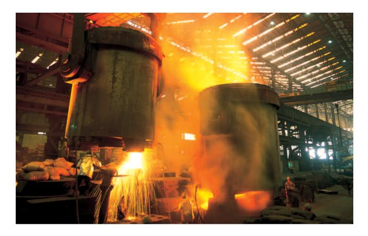
Doosan's steel foundry consists of steel-making and casting shops. The steel-making shop equipped with electric arc furnaces and ladle furnaces has a simultaneous tapping capacity of 700 tons and annual production capability of 260,000 tons of molten steel. This line also has vacuum stream de-gassing equipment to produce heavy ingots for forging and vacuum oxygen de-carburizing equipment for stainless steel.
