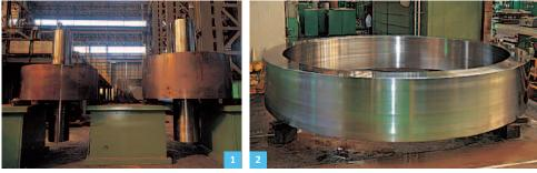
Assembly of Roller & Roller Shaft
