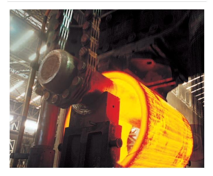
As power plant equipment increases in capacity and is placed under more severer operating conditions, steel castings and forgings for power generation applications are accordingly becoming larger in size and higher in quality.
