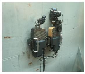
Dome CLP Automated inspection system with remoted vehicle & laser tracker for Dome containment liner plate
