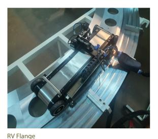
Laser scan and eddy current inspection to maintain the RPV mating surface integrity, to prevent seal leak during operation
