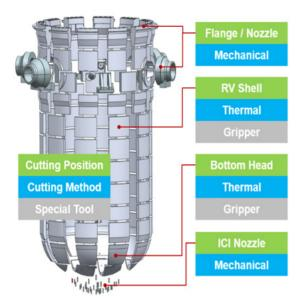
Cutting Plan & Cutting Method for RPV(PWR)
