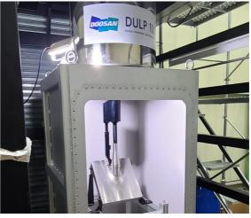
Laser Peening Underwater laser peening system to mitigate tensile residual stress of nozzle and J-weld surface for BMI nozzle
