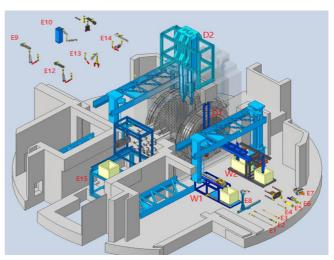
Design of Dismantling Equipment for Radioactive Structures (PHWR)
